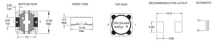
Dimensions are in millimeters.
